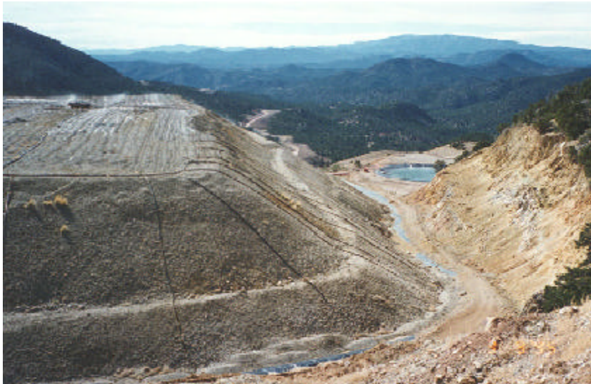
Figure 1.10: The ore is placed on a liner and the solution percolates through the pile. Goldstrike Mine.
