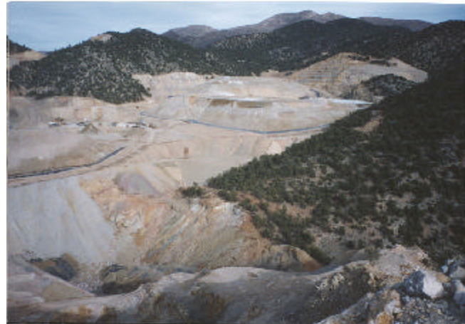
Figure 1.3: A gold heap leach operation will generate large amounts of excess material. Goldstrike Mine.
