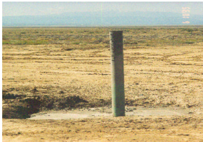
Figure 1.18: Plugged and abandoned well marker.
